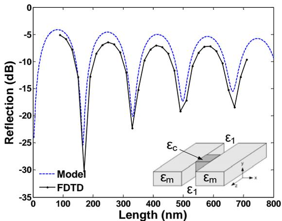
Fig. 5: Reflected power from a Fabry-Pert structure at  $\lambda=1.3\mu\text{m}$  as a function of the length of the silicon core section.
