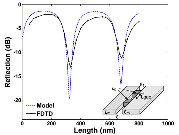
Fig. 7: Reflection spectrum of two coupled Fabry-Pert resonators at  $\lambda=1.3\mu\text{m}$  as a function of their separation distance  $L_{gap}$ .
