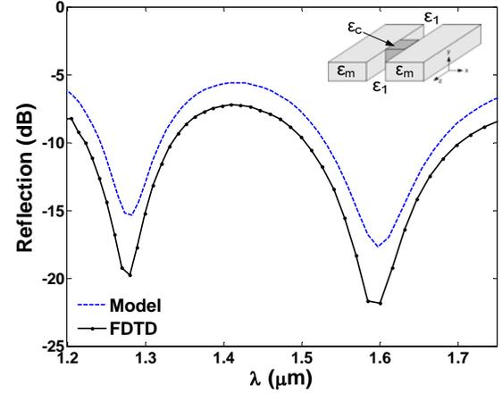
Fig. 6: Reflection spectrum of a Fabry-Pert resonator for a length of  $650\text{nm}$ .
