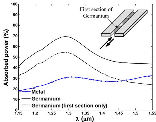
**Fig. 10: Absorbed power in the asymmetric Fabry-Perot photodetector. (The germanium loss is taken as that at 1.3μm.)**
