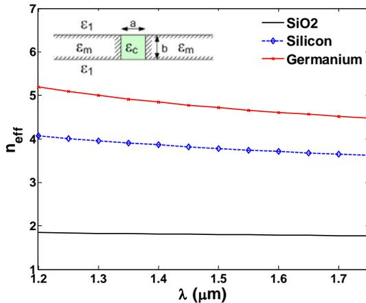
**Fig. 2: Effective refractive index for different filling materials in the core. The inset represents the cross section of the slot waveguide structure. The core region has permittivity  $\epsilon_c$ . (The germanium loss is taken as that at  $1.3\mu\text{m}$ .)**
