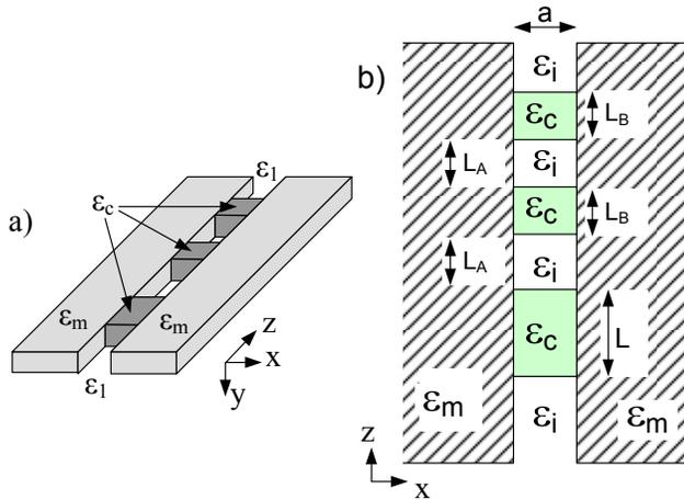
**Fig. 8: Asymmetric Fabry-Perot structure. a) Perspective view. b) Top view.**
