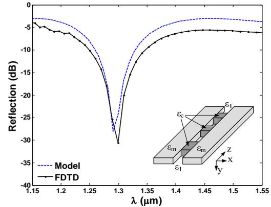
**Fig. 9: Reflection at the front surface of an asymmetric Fabry-Perot structure for a photodetector length  $L$  of  $260\text{nm}$ .**
