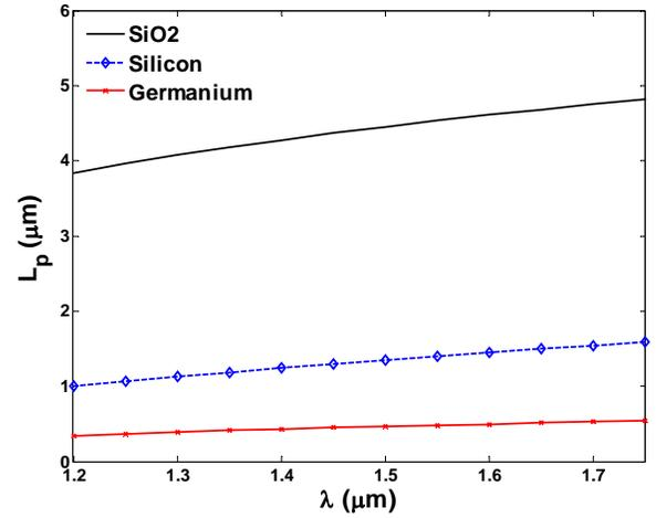
**Fig. 3: Propagation length for waveguides with different filling materials in the core. (The germanium loss is taken as that at  $1.3\mu\text{m}$ .)**
