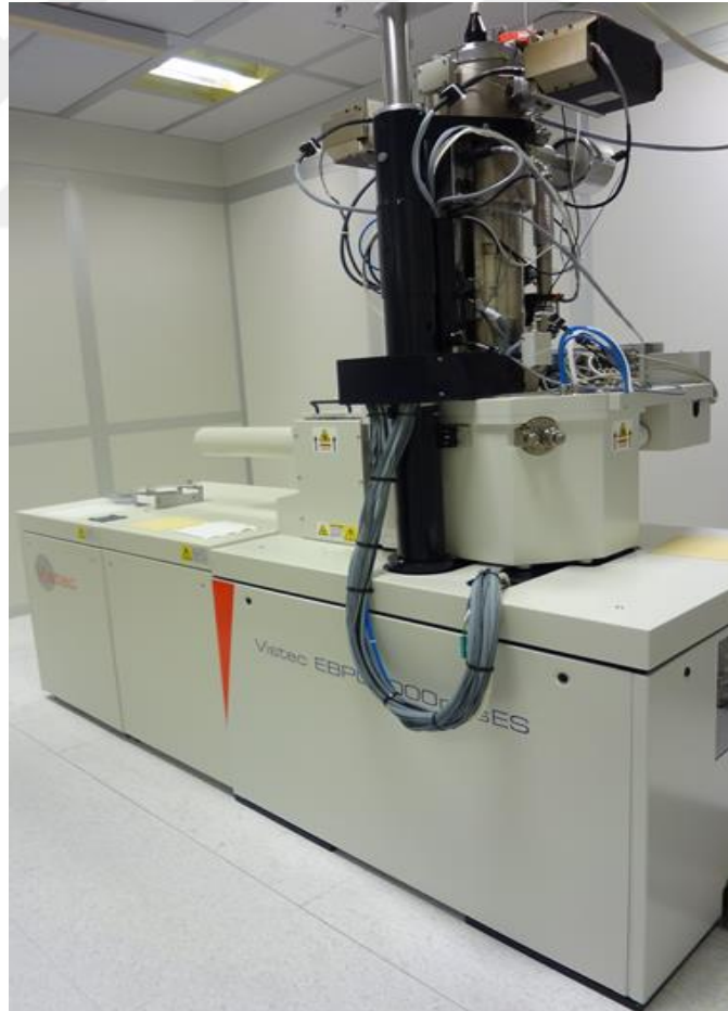
Figure 1.5 Electron Beam Pattern Generator EBPG (Vistec EBPG 5000PlusES).
