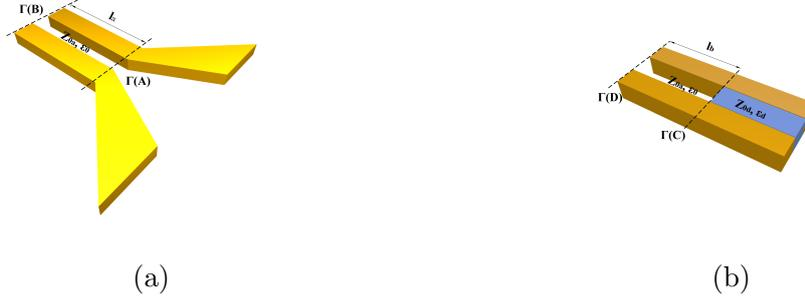
Figure 4.2: Analytical model for impedance matching. (a) Ag-air-Ag TWTL with plasmonic horn. (b) Ag-air-Ag TWTL cascaded with Ag-dielectric-Ag TWTL.
